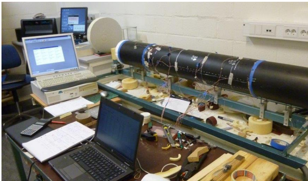
Figure 1. The experimental setup for measuring the temperature profile of the twin district heating pipe.
