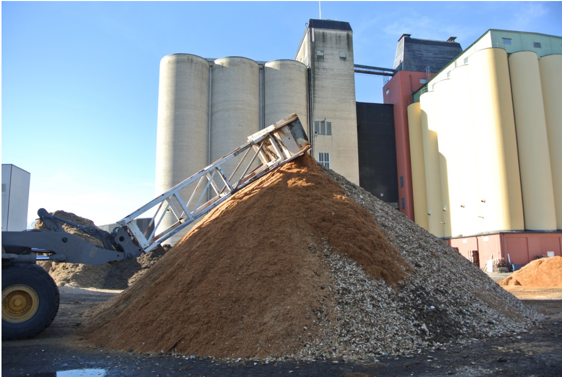
Figur 6. Stackning med stackningsbom Figure 6. Adding a thin layer of sawdust to the pile surface.
