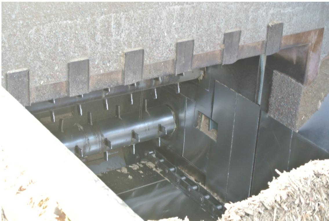
Figur 11. Mottagningsfickans utlopp med två rivarvalsar. Figure 11. Outlet from the receiving pocket with two spike roller.
