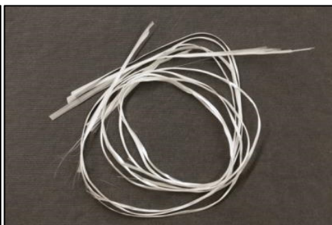
Figure 2 Roving, kontinuerlig fiber
