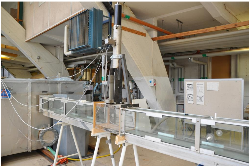
Figure 3 Control valve of knife type of the rig and pressure taps position.
