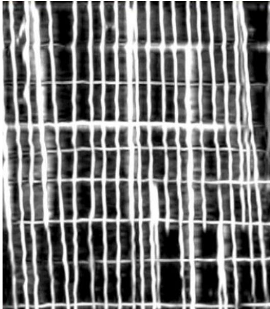
Figure 8: Examples of combined radar scan lines (3D measurements). Measurements at a section of the containment at Barsebäck 1.
