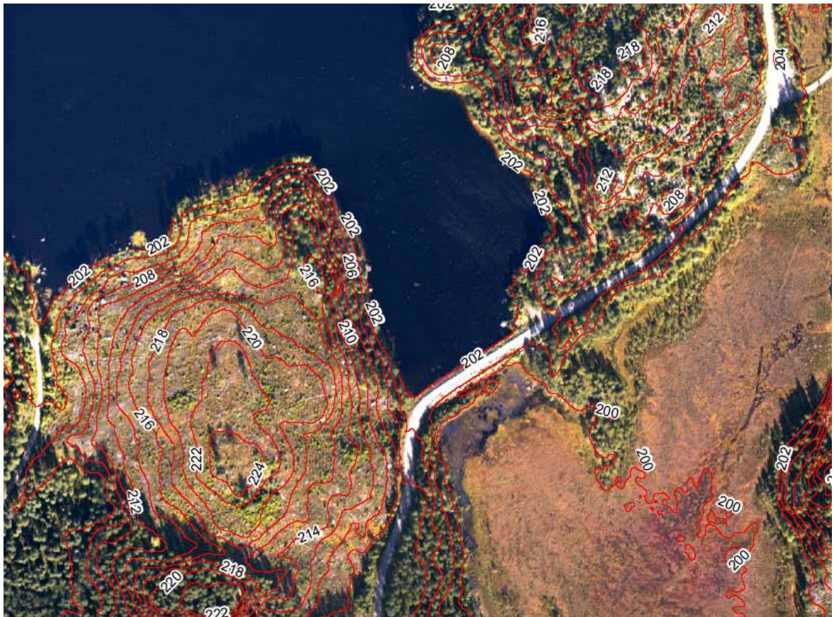
Figure 3-7. 2 m elevation curves from LIDAR superimposed on a co-registered aerial photograph.
