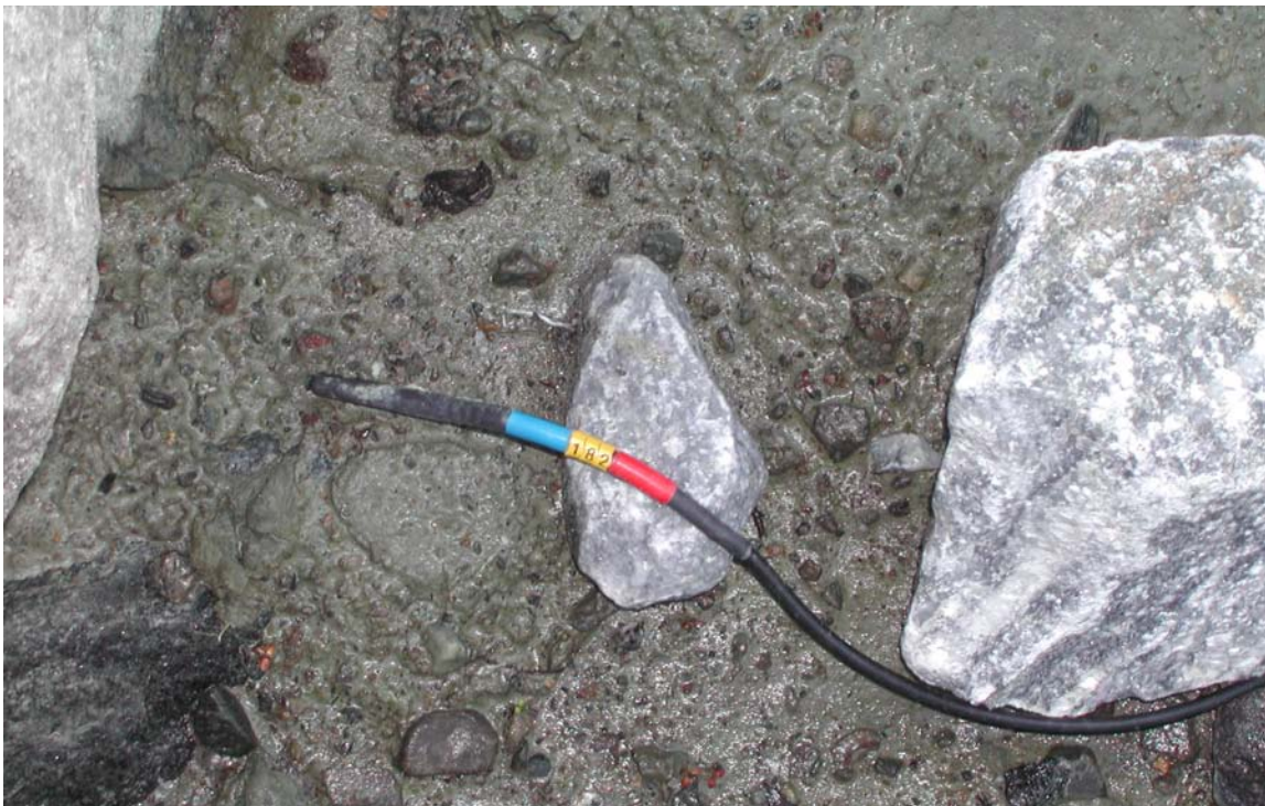
Figure 8-1 Temperature sensor before installation in the soil.
