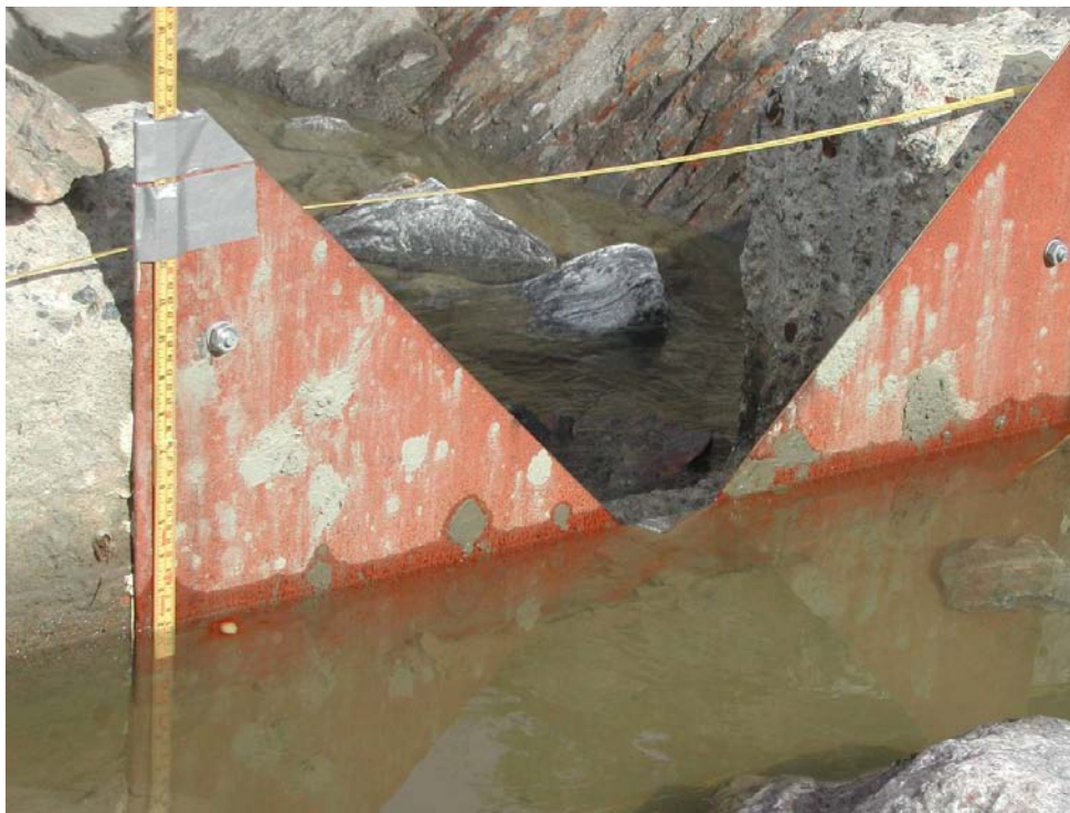
Figure 10 Weir where the seepage flow during the test was measured manually.
