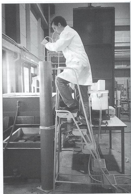
Fig. 2 – Plunge test (CRD C61).
