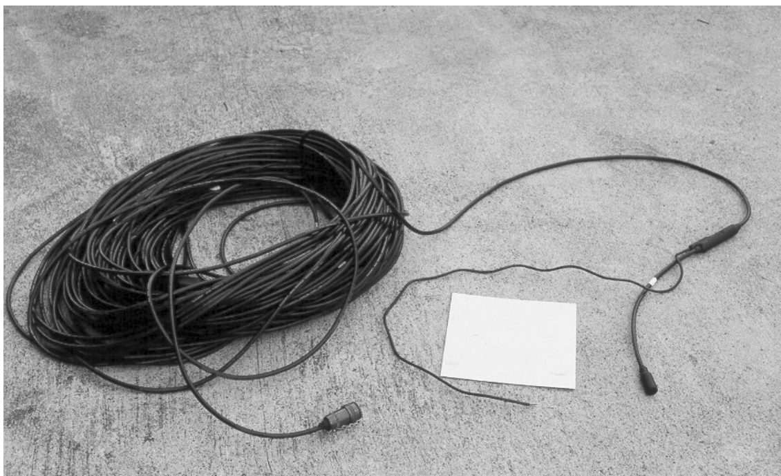
Figure 6 Electrode and multi-core cable used on the dam crest and the downstream toe.
