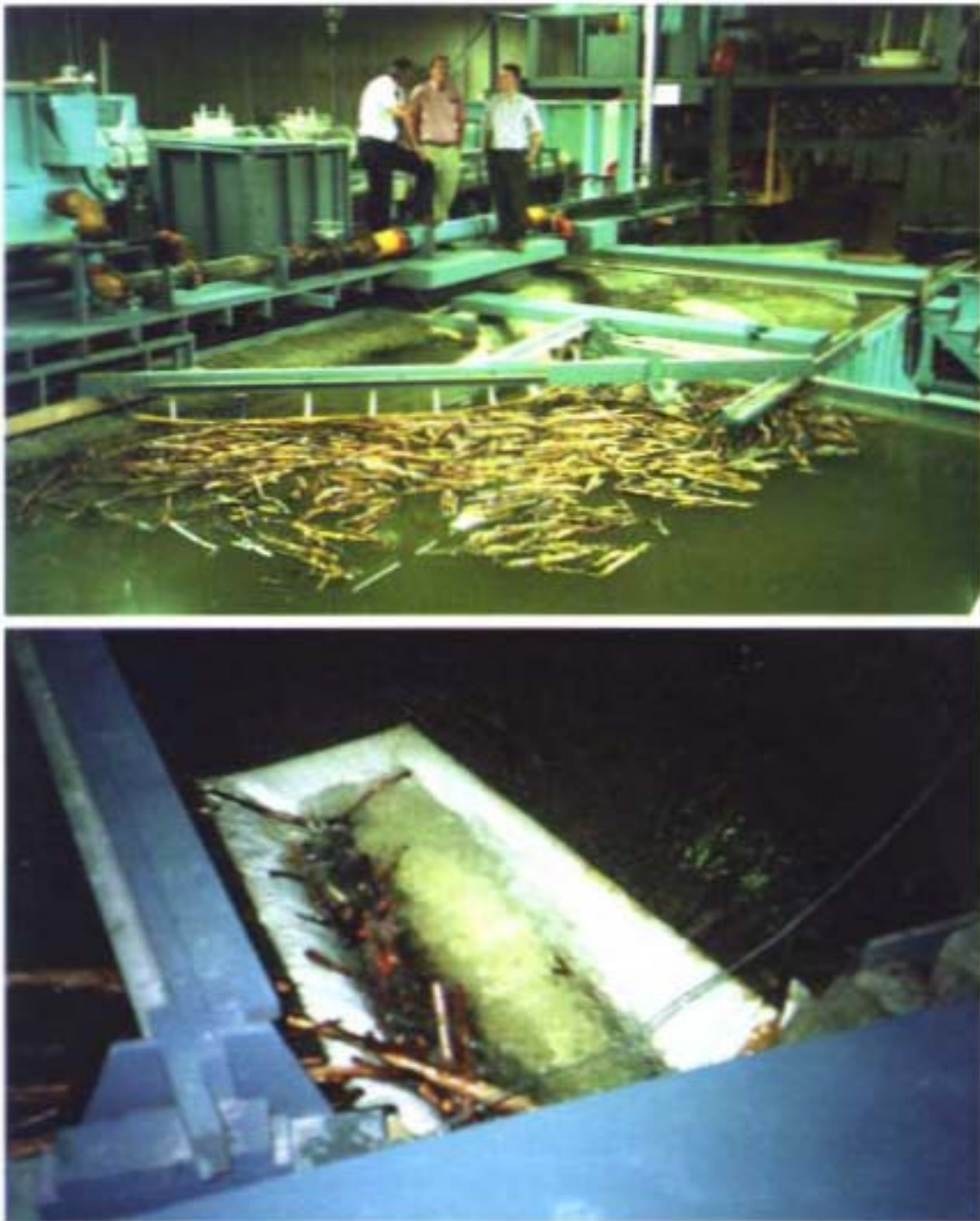
Figure 3.11. Test with floating debris (Canada).
