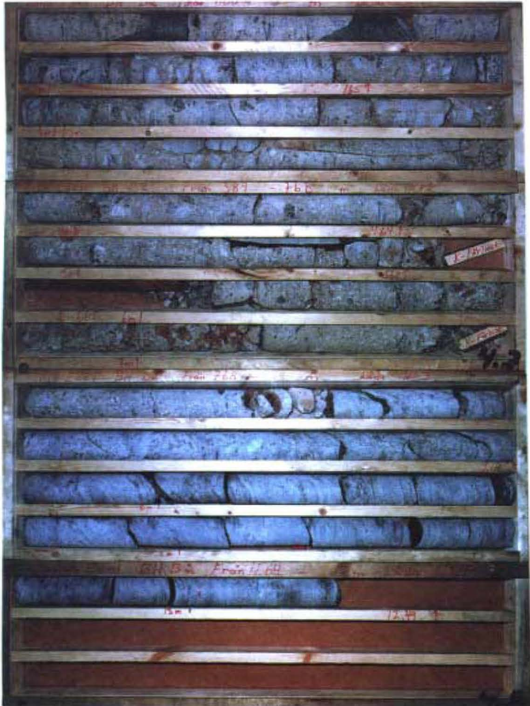
Figure 8.4. Sampling with a core drill gives an idea of the concrete in the structure.
