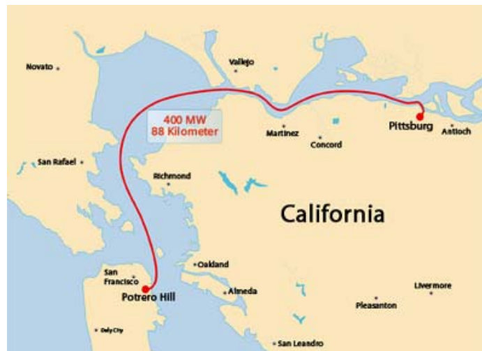
Figure 6.6: The Trans Bay HVDC Link
