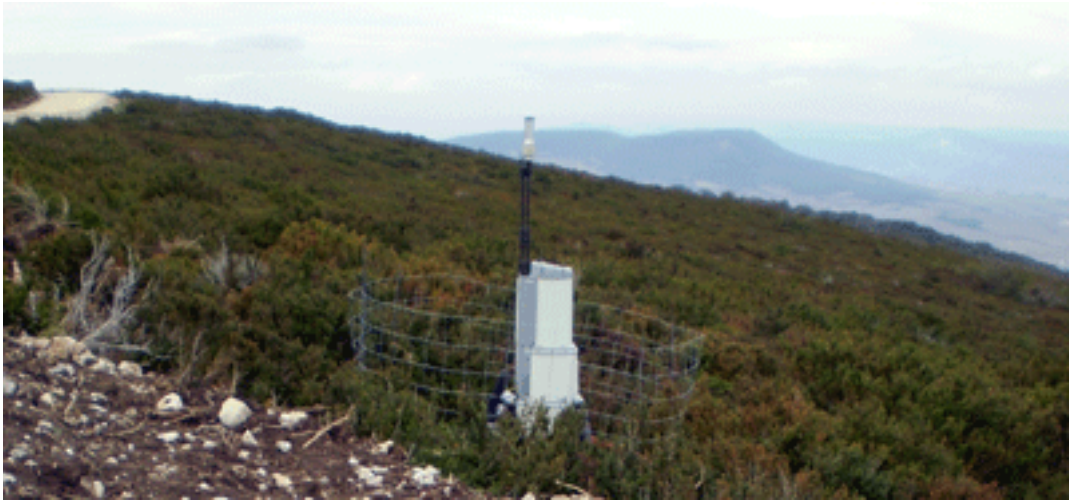
Zephir lidar, total height ca 2 m.
