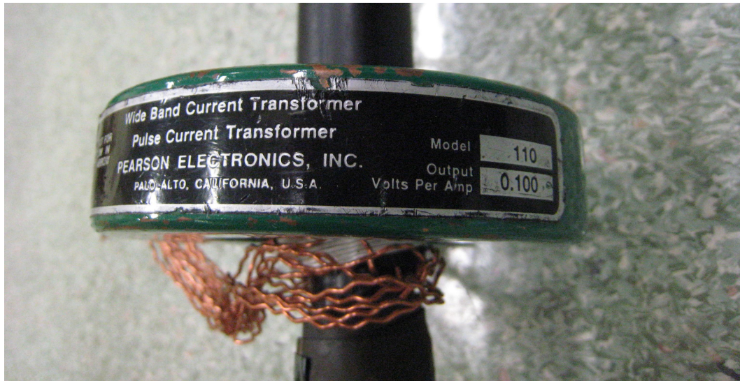
Figure 90 Current measurement device used in laboratory experiment
