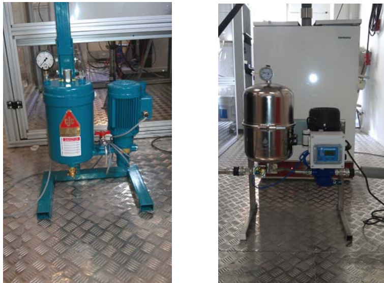
Figure 31. Filter system from CJC (left) and Europafilter (right).
