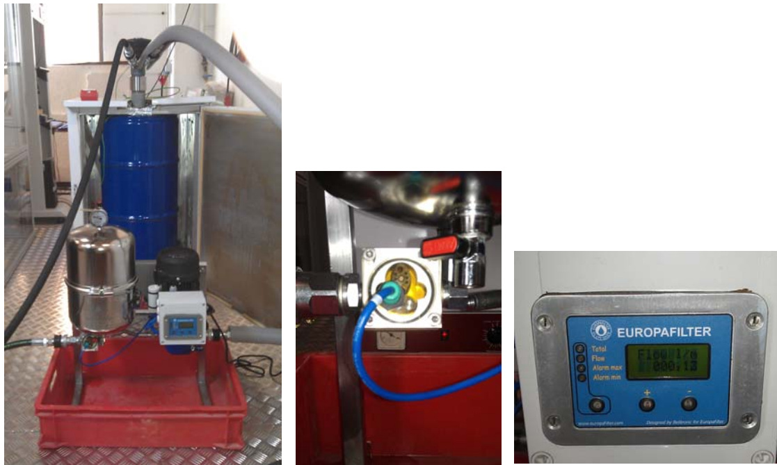
Figure 32. General test design (left), oil flow sensor (middle), data panel (right)
