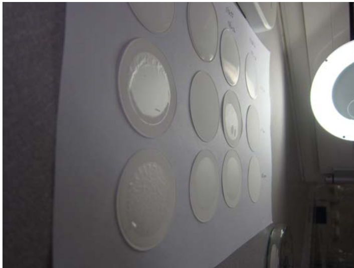
Figure 18. Plastic like shiny layer formed on gravimetric filters.
