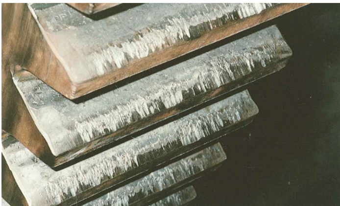
Figure 4. Example of scuffing of gear [2].
