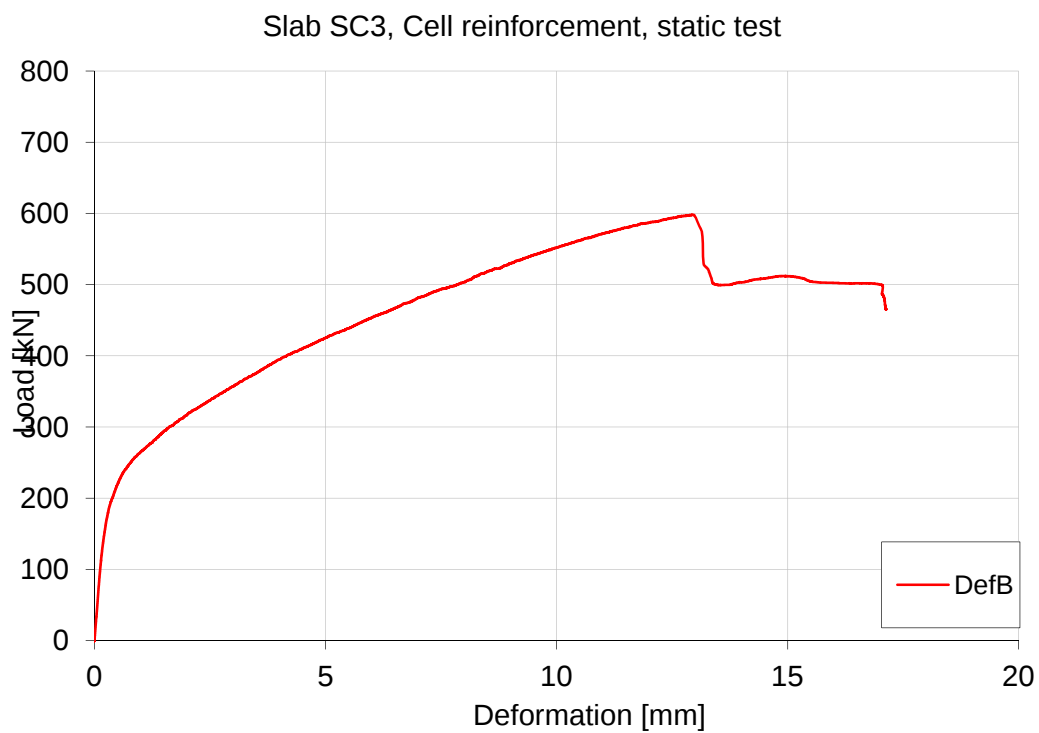
Figure 30 Load – deformation (in the middle) for static failure test of slab SC3.
