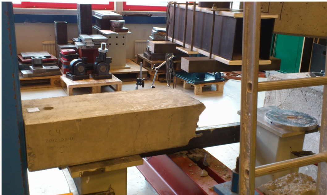
Figure 23 Photo of beam BC4 after testing.
