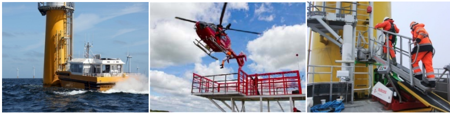
Figure 4-1: Example of transportation solutions for offshore wind farms. Left: Crew transfer vessel , middle: Helicopter hoisting ( http://www.uni-fly.dk ), Right access system for CTV ( http://www.osbitpower.com )
