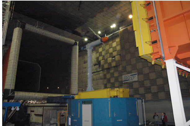
Figure 9.2: Set-up of the Mexico turbine tested in the DNW wind tunnel.
