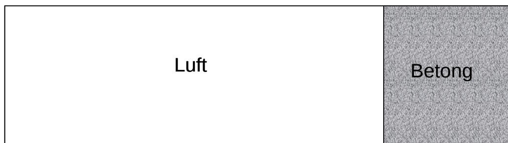
Figur 3.2.1 Geometrisk modell i Comsol Multiphysics.
