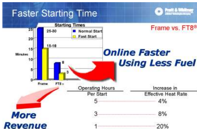
Figure 10-6. Start time influence on engine performance (Courtesy of Pratt & Whitney).
