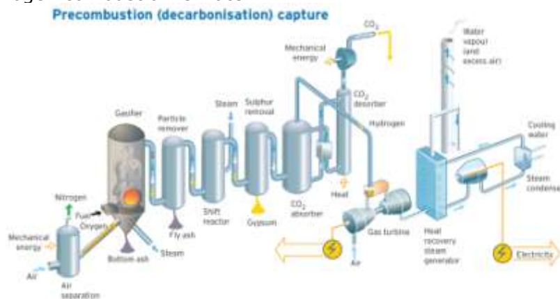
Figure A2-3. Pre-combustion capture technology, source Vattenfall.
