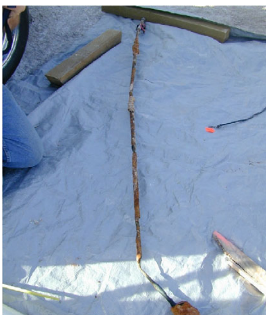
Figure 1. 3/4" x 10' galvanized rod removed after 10 years (Pawnee Site)
