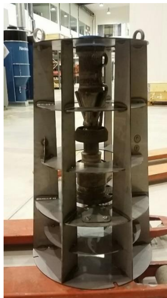
Figure 28. Burner and fixture prepared for spraying
