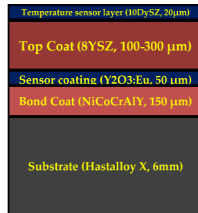
Figure 29. Multilayered TBC system for temperature measurements on the burner
