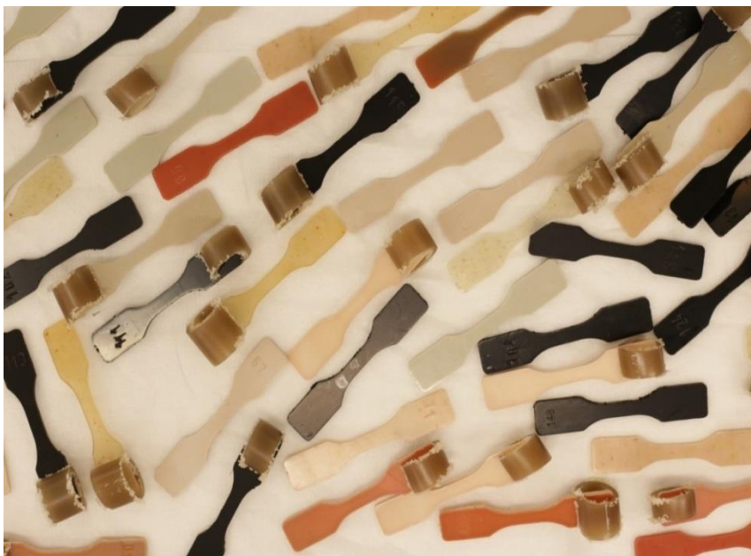
Figure 39. A photo of some of the samples after exposure to 25 wt-% HCl at 60°C for 48 days.
