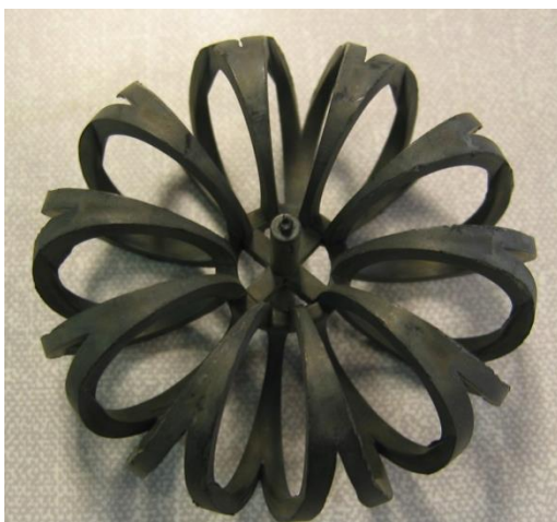
Figure 54. An ADIOX® structure pack filled with active carbon to adsorb dioxins.
