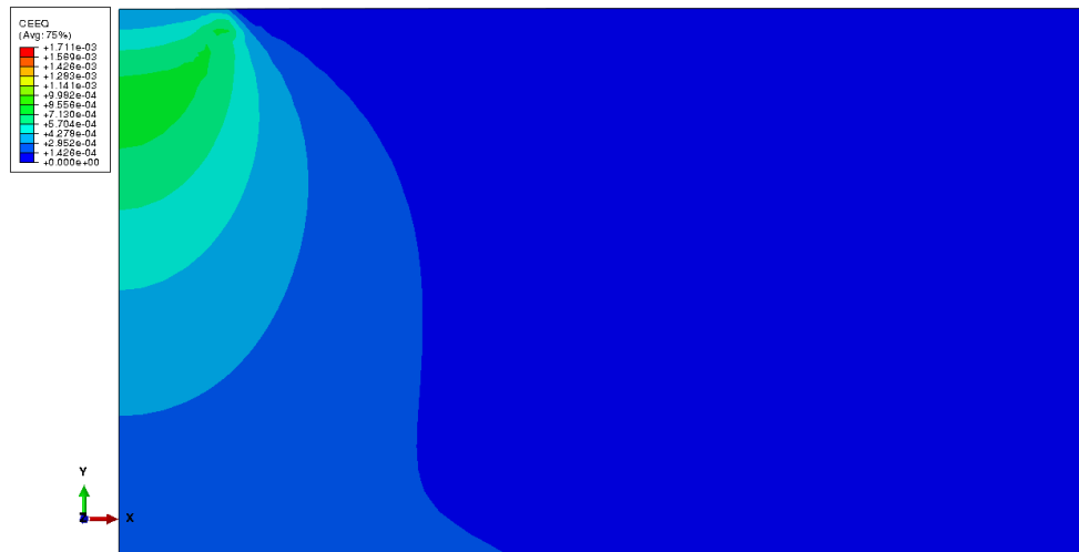
Fig. C3. The equivalent strain distribution in the 2.5mm thick specimen.
