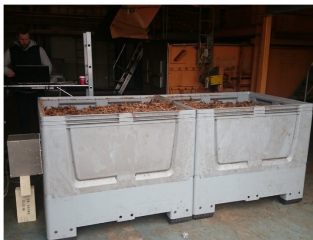
Figure 11. a) Two test boxes of 800 liters and 120x100 cm. Two boxes in a row are 240 cm.
