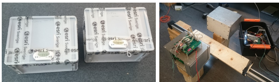
Figure 7. a) Boxes with thermometers. b) Radar scanning of boxes.
