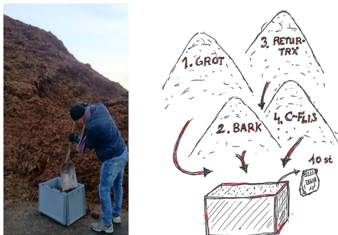
Figure 1. a) Packaging of wood fuel at Gävle Energi. b) Different kinds of fuel have been packaged in the sample boxes and then dried in paper bags or aluminum boxes.
