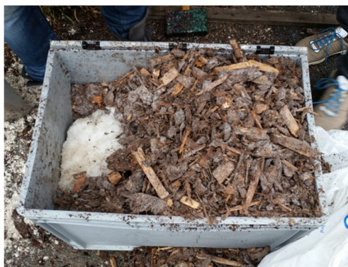
Figure 10. a) Test box with frozen GROT (-18°C) and lump of snow.
