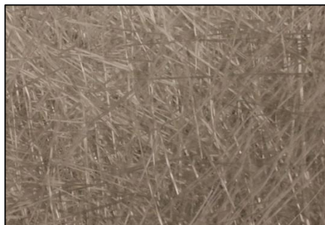
Figur 2 Chopped Strand Mat, CSM
