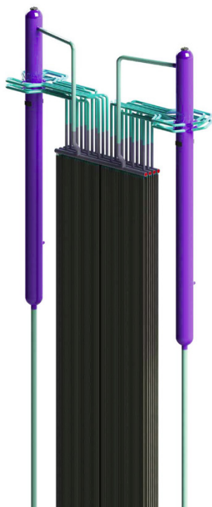
Figure 10-20. Babcock & Wilcox drum attachment design (Courtesy of Alstom)
