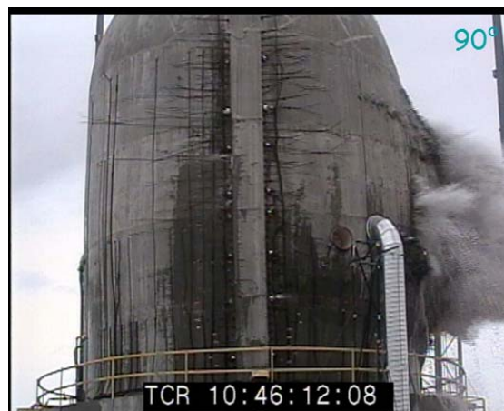
Fig. 6 Pre-stressed concrete containment failure test [SANDIA2006]
