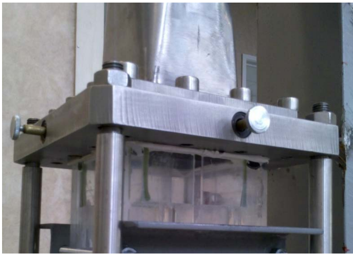
Figure 4: Upper fixation with four ball tip set-screws at 90^\circ
