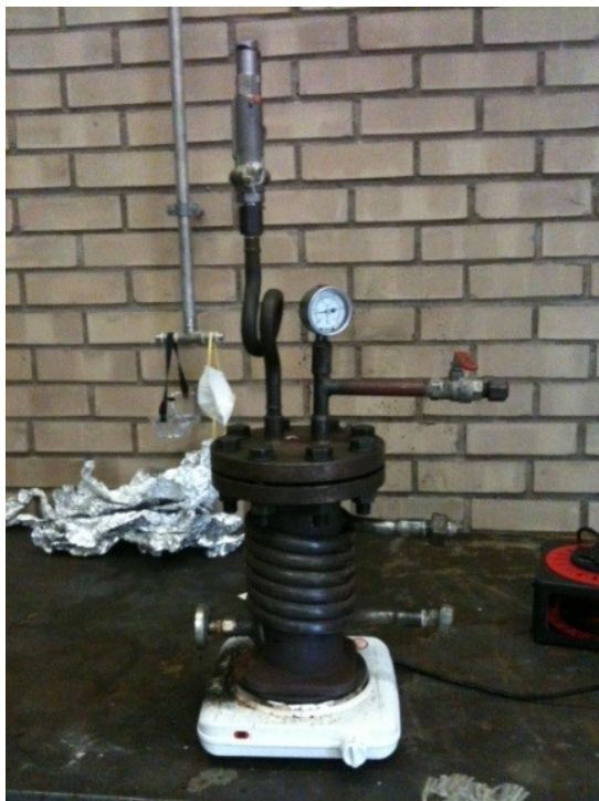
Figure 1: The autoclave used as the HTC reactor for hydrothermal carbonisation of digested sewage sludge from Käppala.
