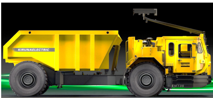
Figur 4 Atlas Copco Electric Minetruck EMT35 (Atlas Copco)
