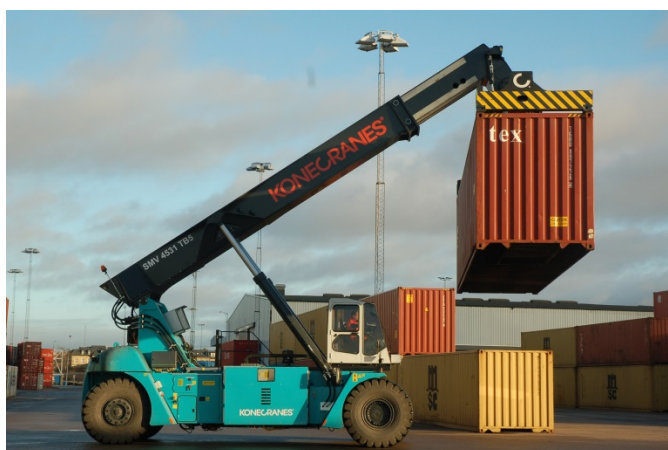
Figur 2 Konecranes hybriddrivna reachstacker (Konecranes, 2013)
