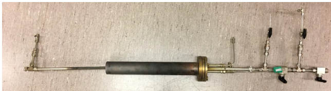
Figure 5: Reactor in the Chalmers laboratory unit
