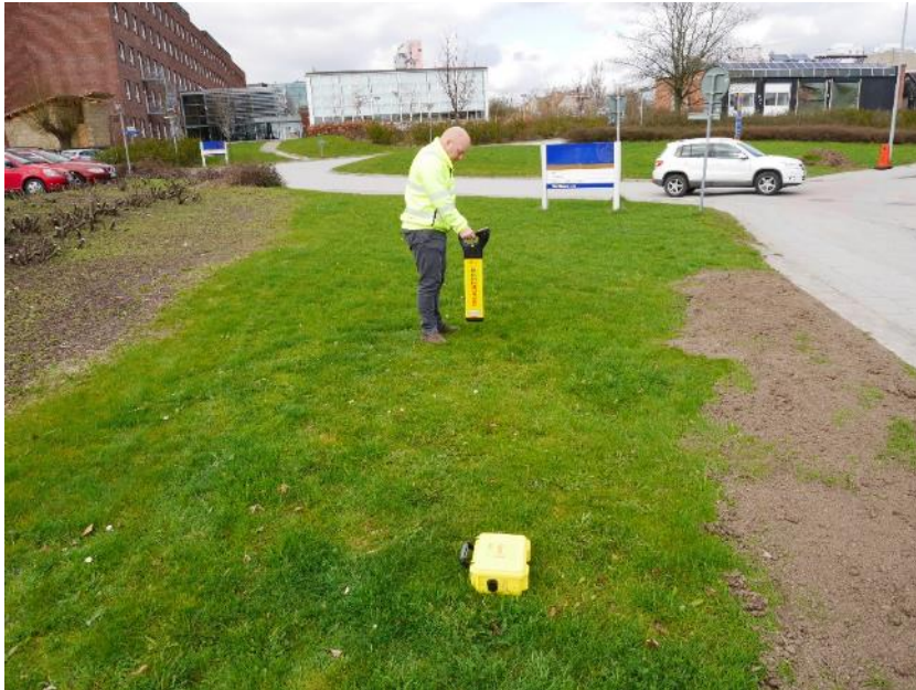
Figure 25. Leica cable-finder system. Near: Digitex transmitter (induction or connection) and Distant: Digicat receiver.
