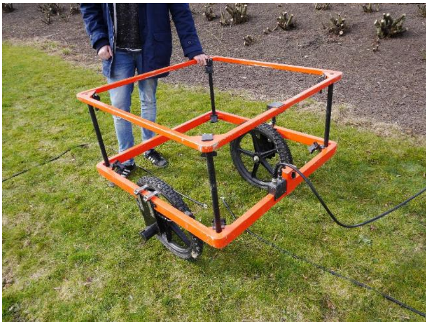
Figure 15. Geonics EM-61 TEM sensor with two different coils. The black cable is the LTH test square.
