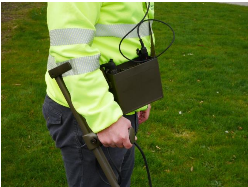
Figure 22. Schiebel AN-19 control unit. Dials for sensitivity and headphone loudness.
