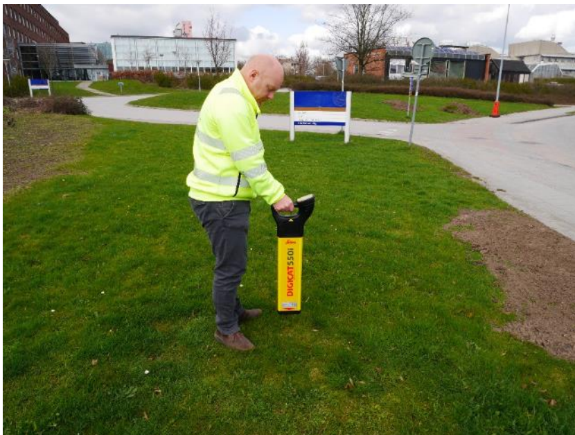
Figure 24. Leica Digicat 550i Cable-finder. Magnetic field detector. Requires current in the cable to be detected.
