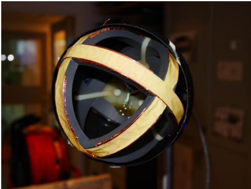
Figure 13. Top of sensor head removed to show the arrangement of the three orthogonal coils.
