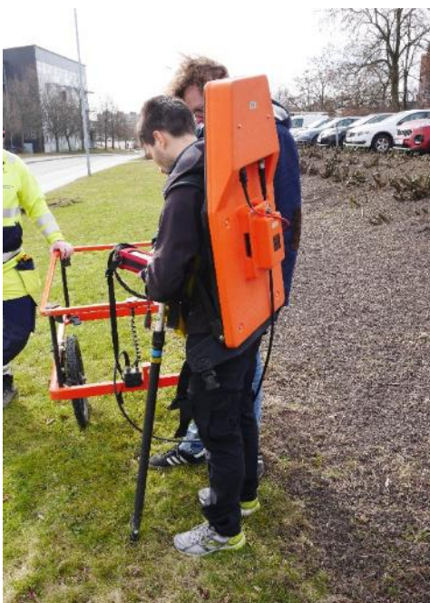
Figure 17. Geonics EM-61 back pack (batteries, power electronics)
