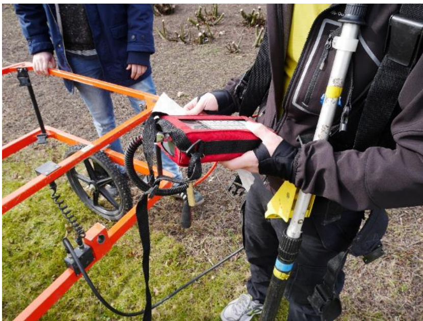
Figure 16. Geonics EM-61 control unit
