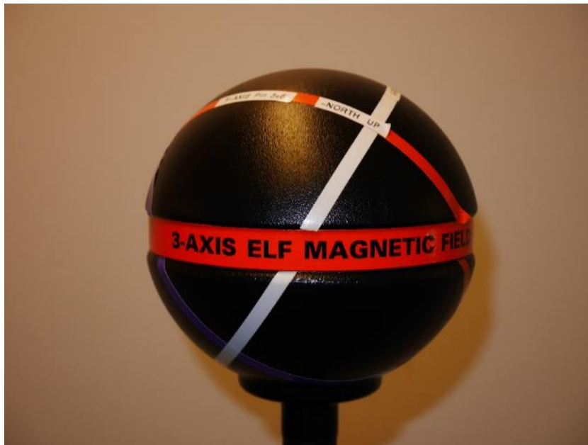
Figure 12. The sensor head of the total magnetic field instrument. Thin lines indicate the orientation of the coils inside the sensor head.
