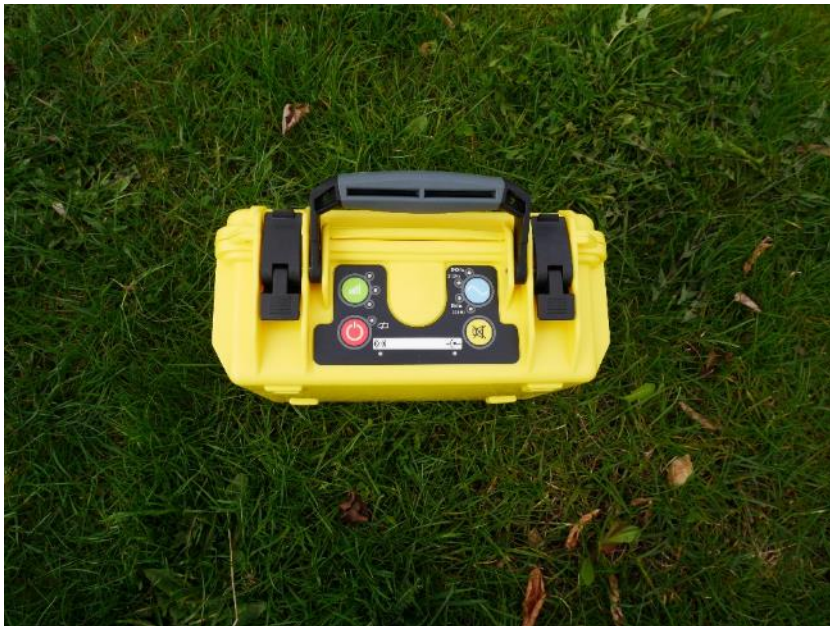
Figure 26. Leica Digitex inductive/connective transmitter for frequencies 8 kHz or 33 kHz.
