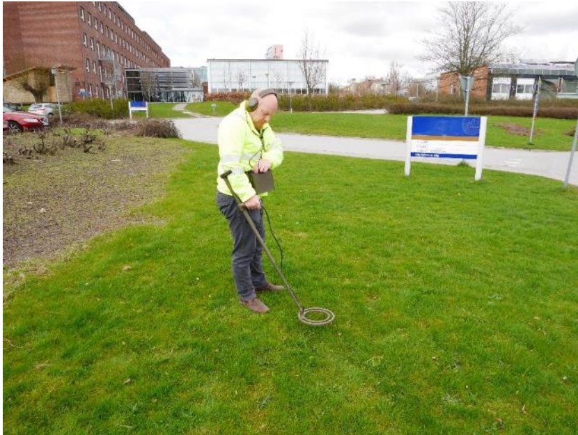
Figure 20. The Schiebel AN-19 military mine seeker (courtesy of FOI)
