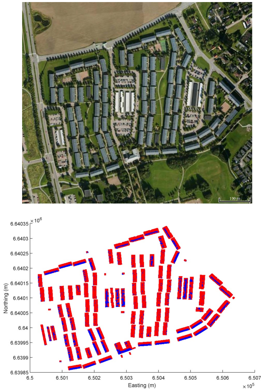
Figure 4. An example of a residential area in Uppsala aerially photographed (above) and represented by the raster based on LiDAR data (below). In the lower subfigure, red and blue cells have annual irradiance below and above 1000 \text{ kWh/m}^2 , respectively.
