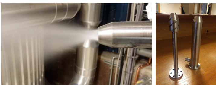
Figure 6: Tar injection nozzles and the spray pattern.
