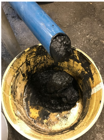
Figure 8: Wood tar feeder outlet.
