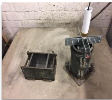
Figure 4.6: Second attempt setup (a) a steel frame (b) fixing steel frame inside the mould and (c) casting concrete
