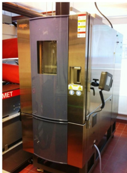
Figure 2.6: Climate chamber connected to the NSI X5000 system.
