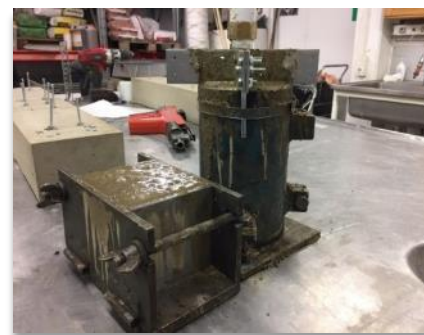
Figure 4.6: Second attempt setup (a) a steel frame (b) fixing steel frame inside the mould and (c) casting concrete
