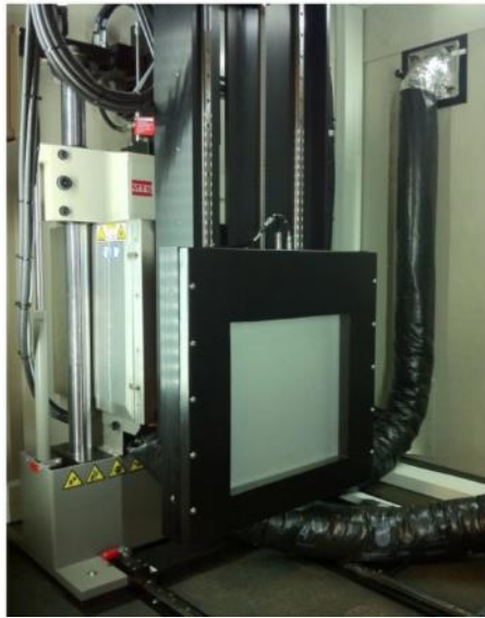
Figure 2.3: Digital detector with 200 mm pixel pitch in the NSI X5000 system.
