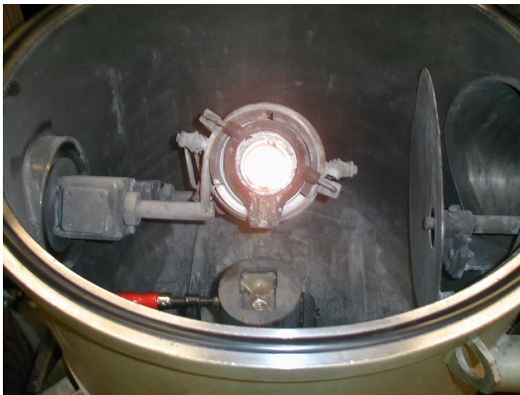
Figure 6: Interior of the induction furnace showing the crucible in the center and the mold below.
