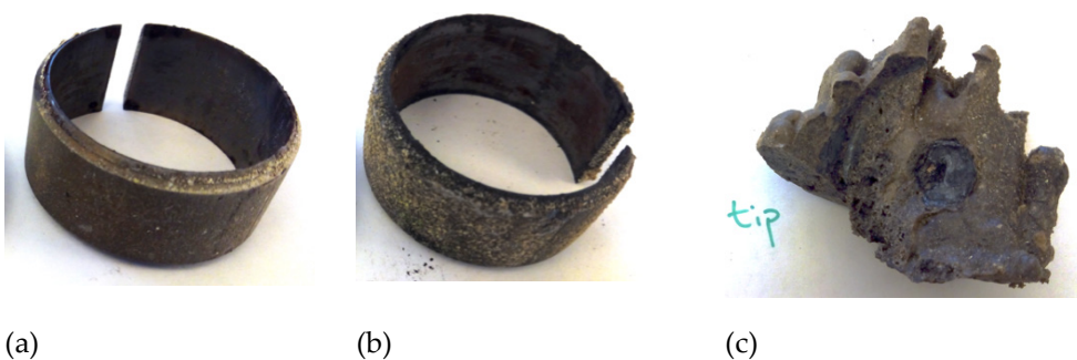
Figure 34. Images of three different deposits after 2 hours of exposures from the settings (a) K22, (b) S22 and (c) C11. 29 different conditions were set up in the boiler in order to find out the less corrosive one. All the deposits from the 29 settings were analysed to select the one to run the corrosion test
