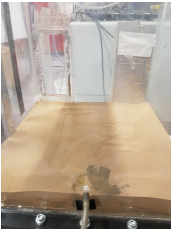
Figure 10: The cold flow model combustor chamber with sand and no fluidization.
