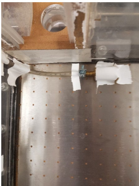
Figure 9: Setup of the hose for extra fluidization shown in the cold flow model combustor chamber when no bed material is added.
