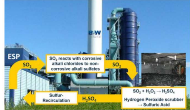
sulphur recirculation in a bio plant
