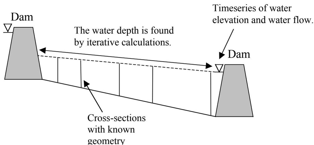
**Figure 2 Simplified representation of the river between the hydropower stations**
