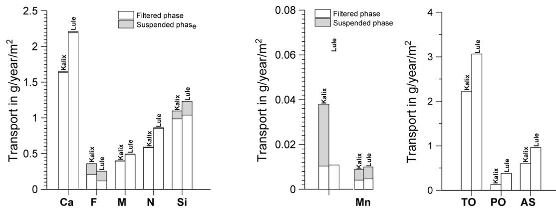
**Fig.13. Annual transport in the Lule and the Kalix Rivers (in g/year/m<sup>2</sup> of the drainage area)**
