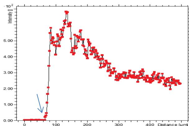
**Figure 9.** ToF SIMS measurement on EPDM where oxidation ( $O^-$  signal intensity) is presented as function of distance from the sample surface-air interface (shown with an arrow) towards bulk material. In this case the ca. 200  $\mu\text{m}$  thick surface layer has oxidized more than the bulk material.
