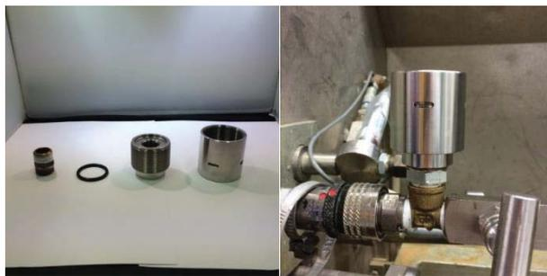
**Figure 2.** The test rig for leakage measurements, to the left before mounting the O-ring and to the right mounted for leakage test. Leakage was detected at the hole in the cylinder. O-rings were exposed to radiation and heat mounted inside the test rigs.
