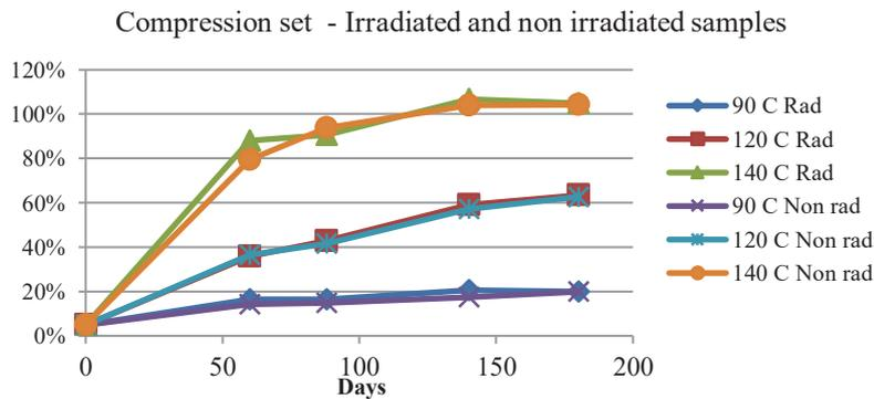
**Figure 3.** Compression Set Measurements for EPDM O-rings with 2,99 mm diameter.
