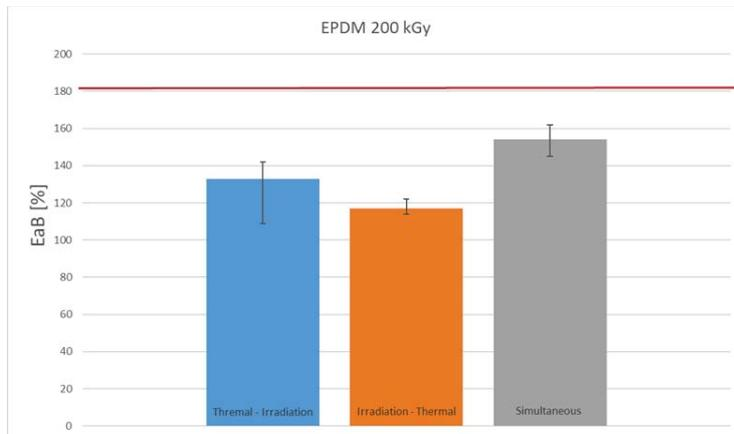
**Figure 8.** Comparison of sequence of ageing on EPDM samples. Blue column describes the decrease in EaB when sequence is thermal-irradiation, orange column irradiation-thermal and grey column simultaneous thermal and irradiation ageing.
