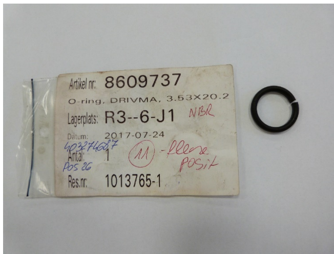
Figure 23: Hard and brittle NBR O-ring (from Ringhals, service conditions unknown).
