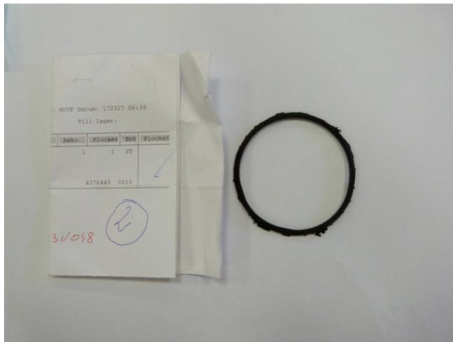
Figure 22: Damaged EPDM O-ring (from Ringhals) after service at 50°C for 6 years.
