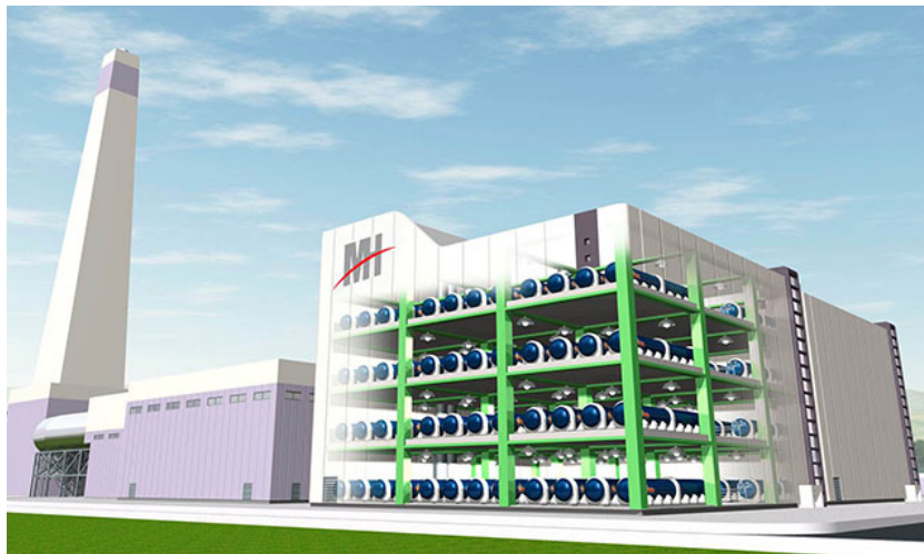
Sketch of planned MHPS Gas Turbine Fuel Cell Combined-cycle Power Plant. Courtesy of MHPS.
