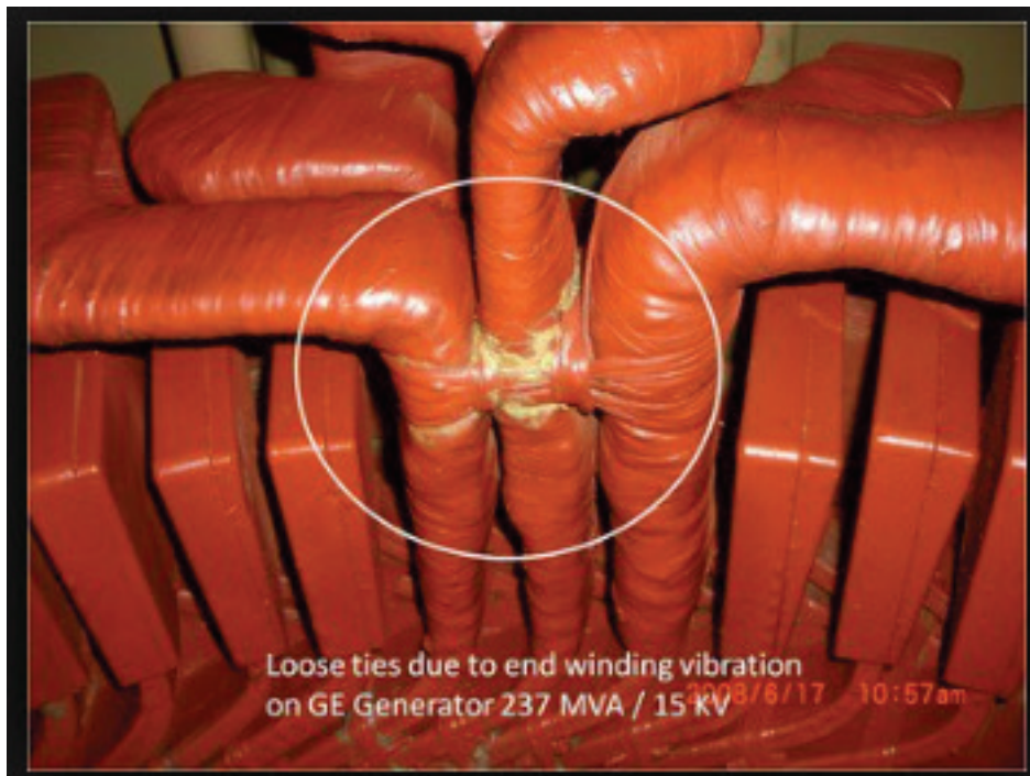
Figure 49. Fretting wear in tied connection points
