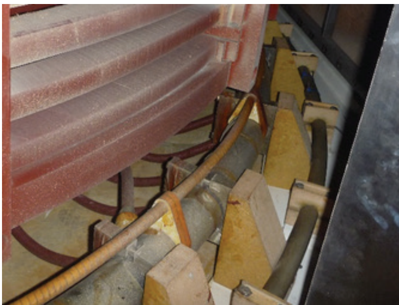
Figure 68. Manifolds with fixation supports
