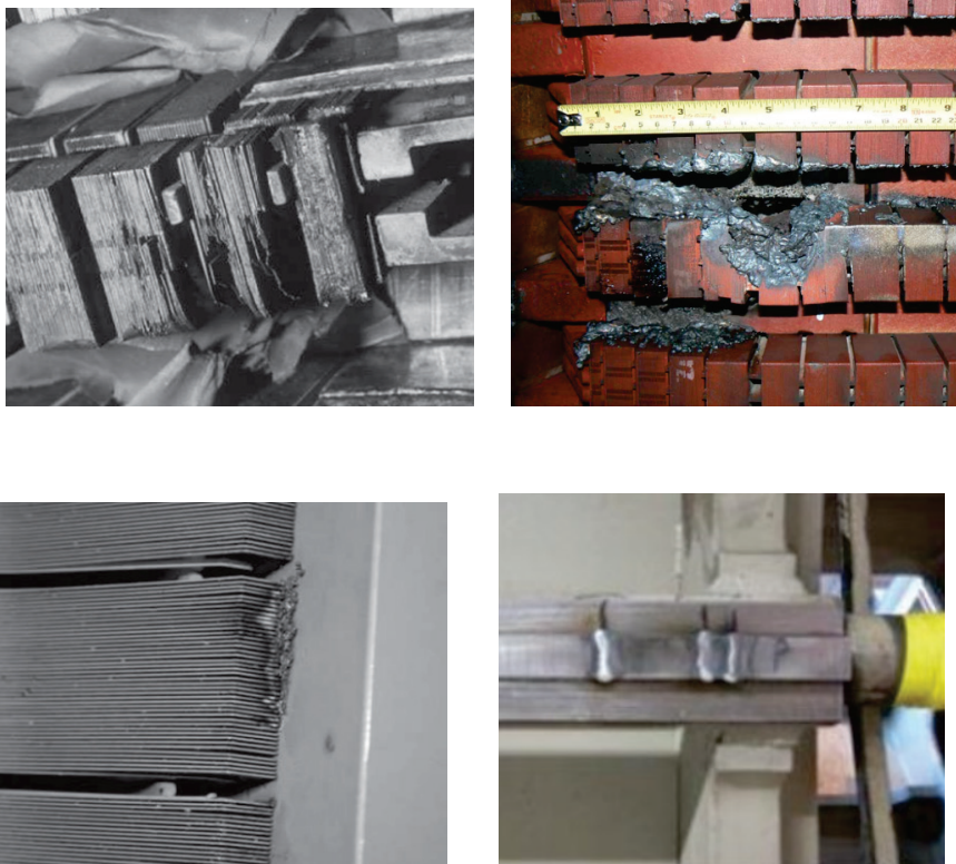
Figure 3. Examples of core failures
