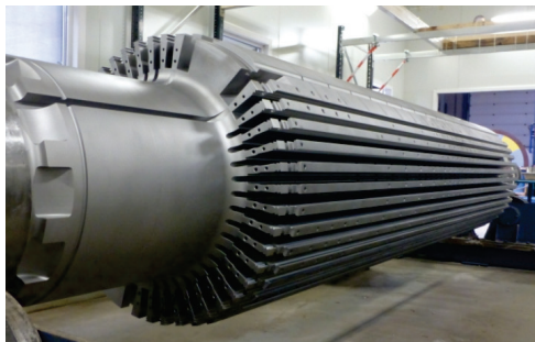
Figure 12. A 2-pole rotor forging in the milling machine
