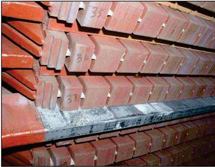
Figure 4. Abrasion from corona and vibrations
