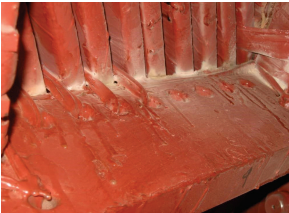
Figure 48. Fretting wear and Abrasion flour in broken contact surfaces
