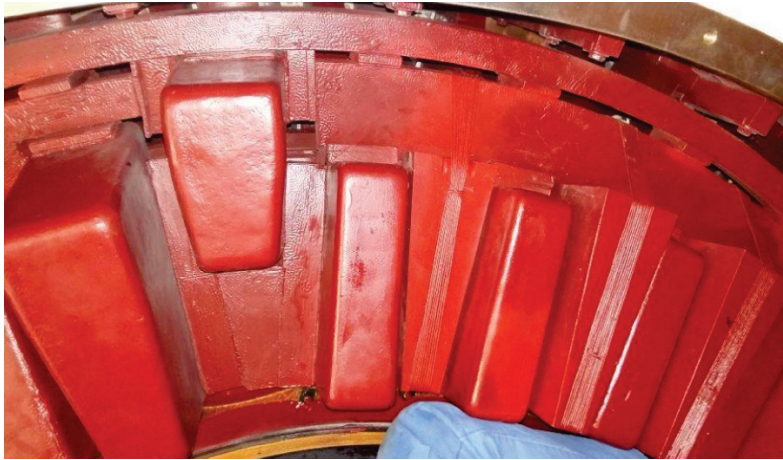
Figure 84. Tuning weights after reconditioning
