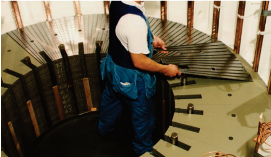
Figure 16. Stacking of core with the use of thin segments
