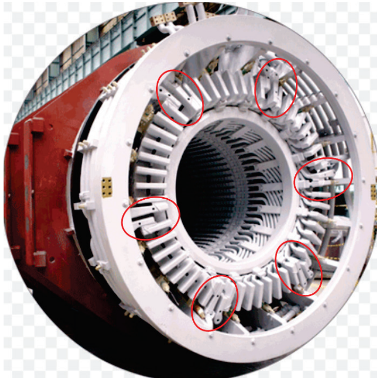
Figure 30. Round connection conductors between winding and round connection marked with red
