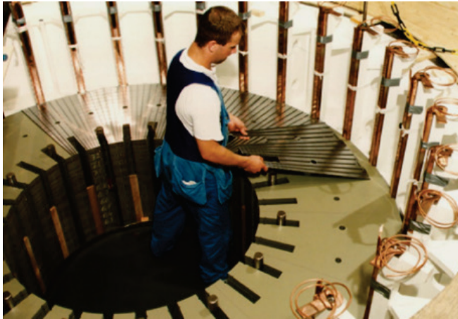
Figure 75. Building bar of copper
