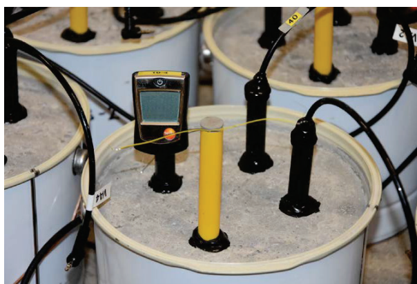
Figure 2-14 – Measurement of borehole, [16]. The RH meter is placed in a drilled hole, where its endpoint corresponds to the position of the object in which the RH is to be determined
