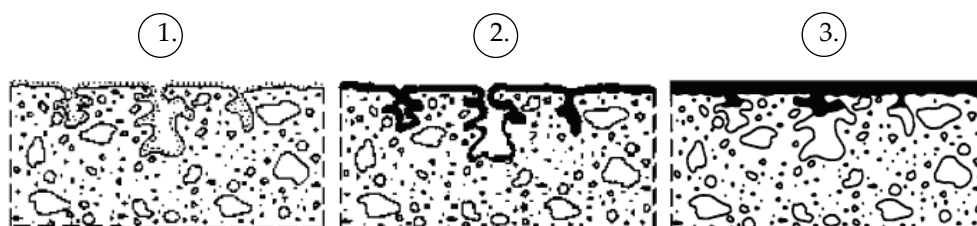
Figure 4-6 (1) Water repellent impregnation. (2) Impregnation. (3) Surface coating
