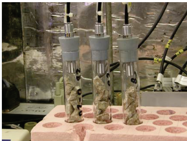
Figure 2-13 – Measurement of RH from samples obtained from the structure. The samples are placed in a test tube and a capacitive RH meter it placed into the tube [16].
