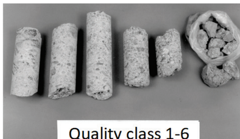
Figure 2-29 – Example of what cores from their respective quality class may look like [36].
