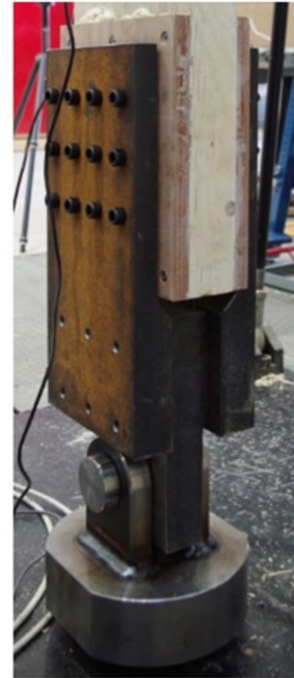
Detail of the reinforced bolted end connection
