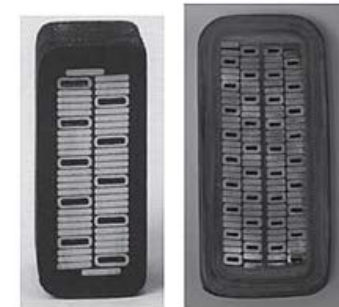
H 2 O-cooled stator bars
