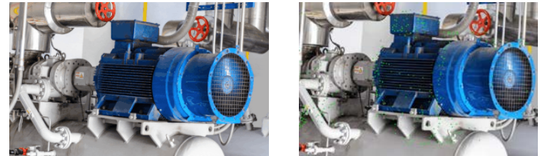
Video Vibration Tracking - DragonVision™ Video Deflection Technology [4]
