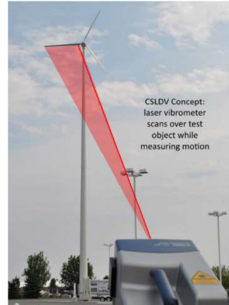
CSLDV Modal analysis of Wind turbine [1]
