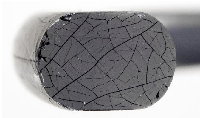
HNBR O-ring after 1 year at 150°C
