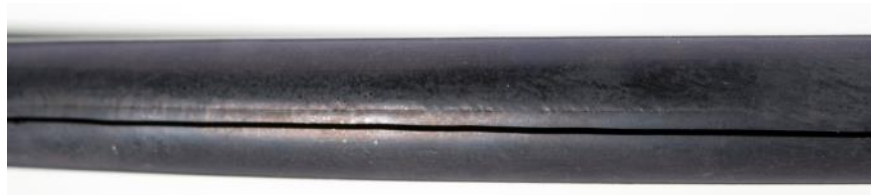
EPDM O-Ring after ageing for 1 year at 150°C
