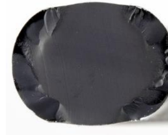
Cut cross-section of HNBR O-ring aged for 100 days at 150°C
