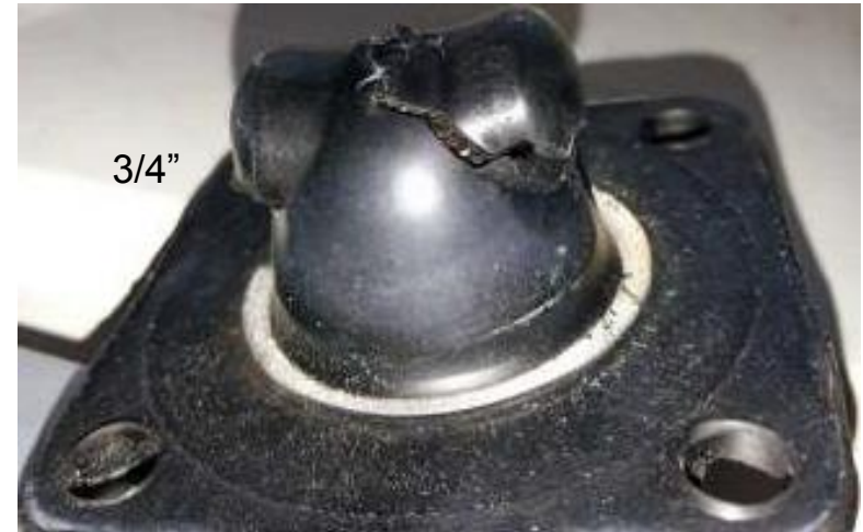
Diphragm from valve 40741V4170 after 20 years in use.
