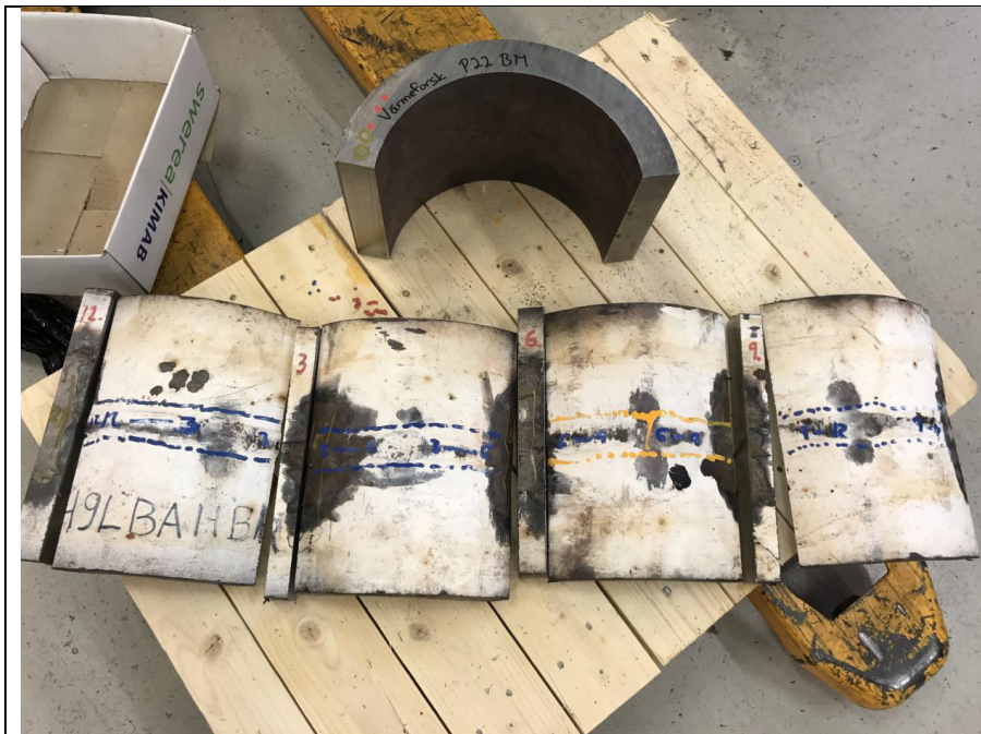
Figure 1. The material received for the testing. In the foreground is the weld, cut up for specimen manufacture. In the back is the material used for new base metal. The material for service exposed base metal came from the rightmost piece, upper part (between clock position 9 and 12).
