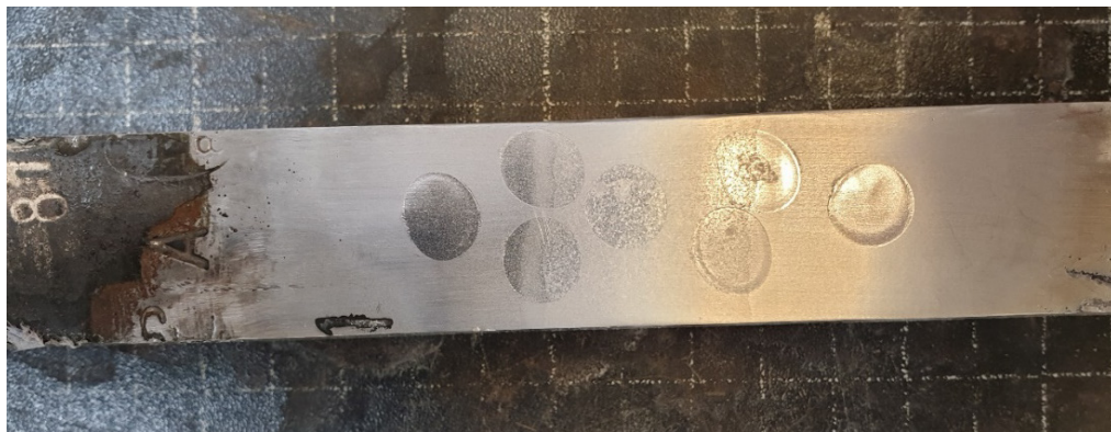
Figure 12. Tested positions along the surface of the weld. Base metal 1 corresponds to the leftmost polish point and base metal 2 the rightmost point.
