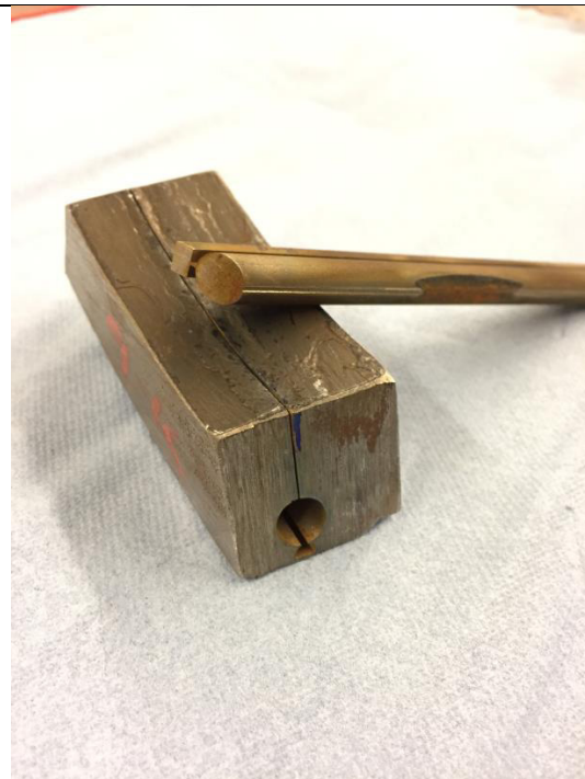
Figure 2. The special geometry used for the weld metal service exposed specimens. Alongside the sound blank a rectangular piece was cut. This was later polished and studied metallographically to assess the creep damage before testing in the specimen gauge.
